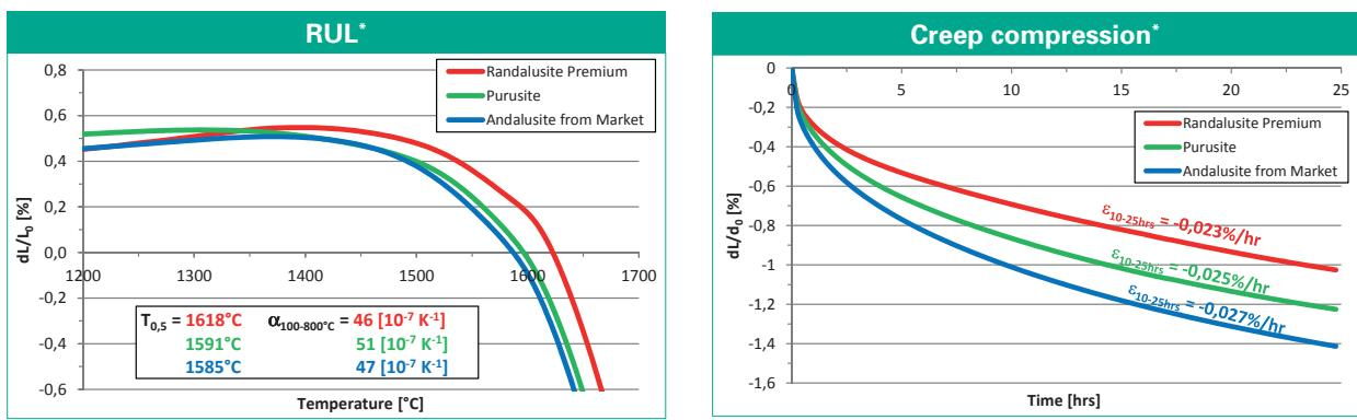
\*Refractoriness under load & creep in compression at 1500°C on bricks according to European standards EN 993-8 and EN 993-9
